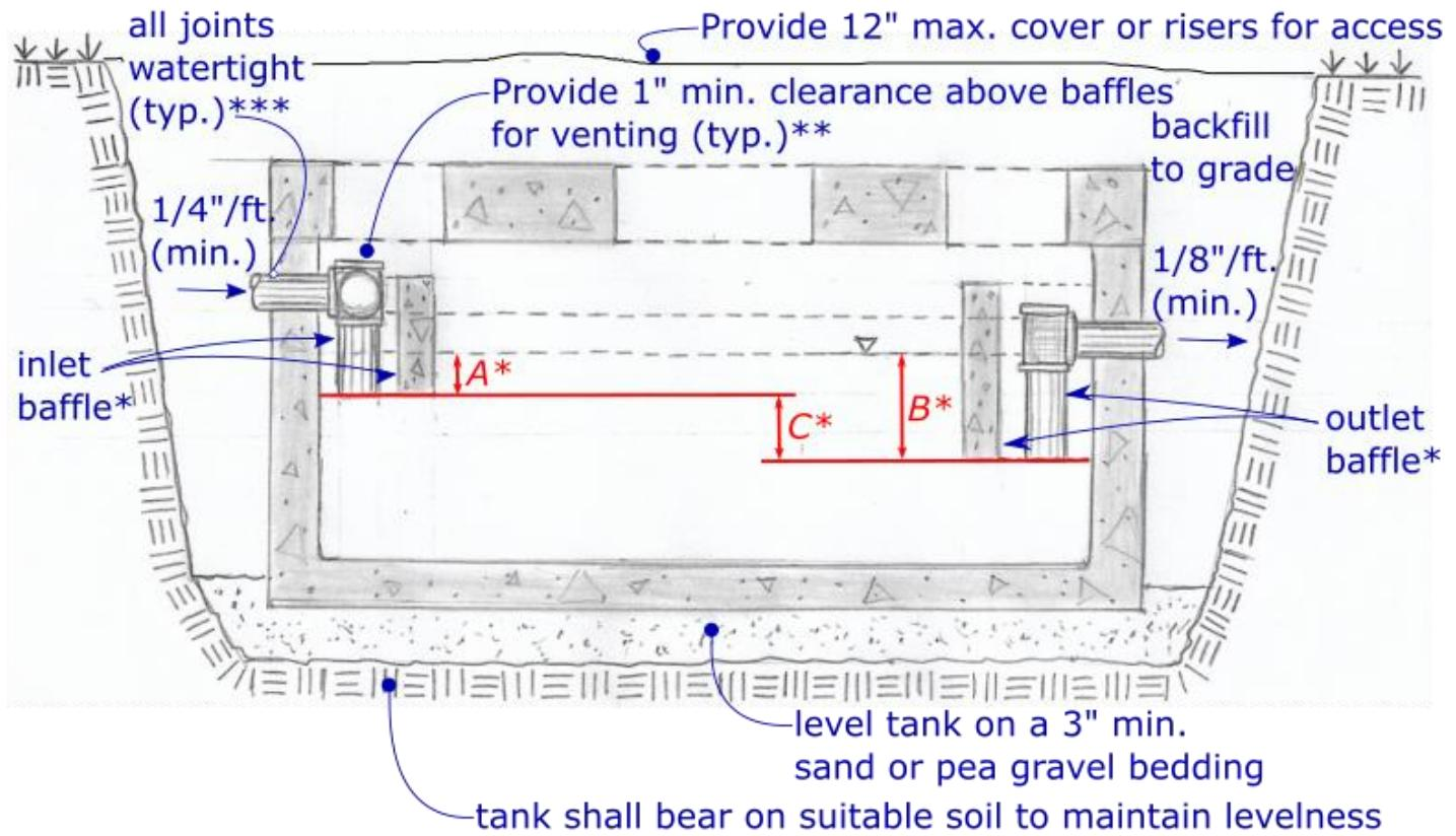
\*baffles may be constructed of pre-cast concrete or piped sanitary tees
