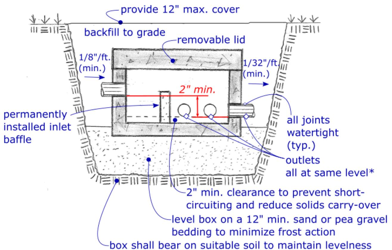
\*Install speed levelers to ensure equal distribution of flow. All unused outlets must be plugged and parged.
