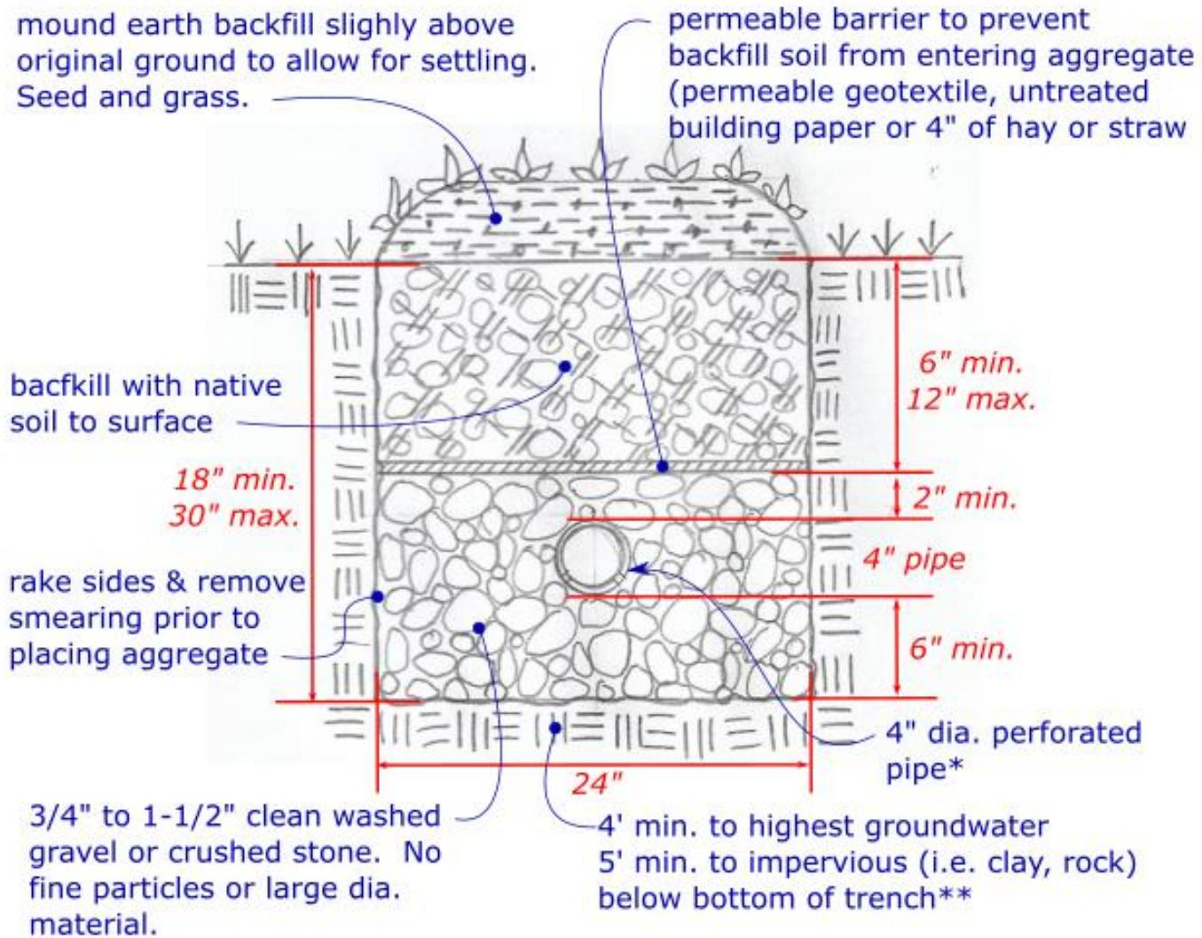
\*Pipe to meet ASTM standards for septic systems and to be installed with perforations facing bottom of trench. Piping shall be installed with a slope of 1/16"/ft. to 1/32"/ft. with capped ends. Pipe lengths determined from Table 4A in Section III and/or accepted SAN36a proposal.
