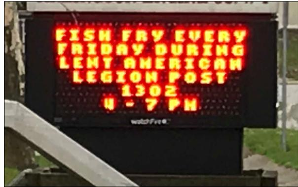
*This digital sign showcases the characteristic "glow" around LED bulbs that can impede legibility. The use of all-caps and wide letter-spacing also makes it harder to read.*
