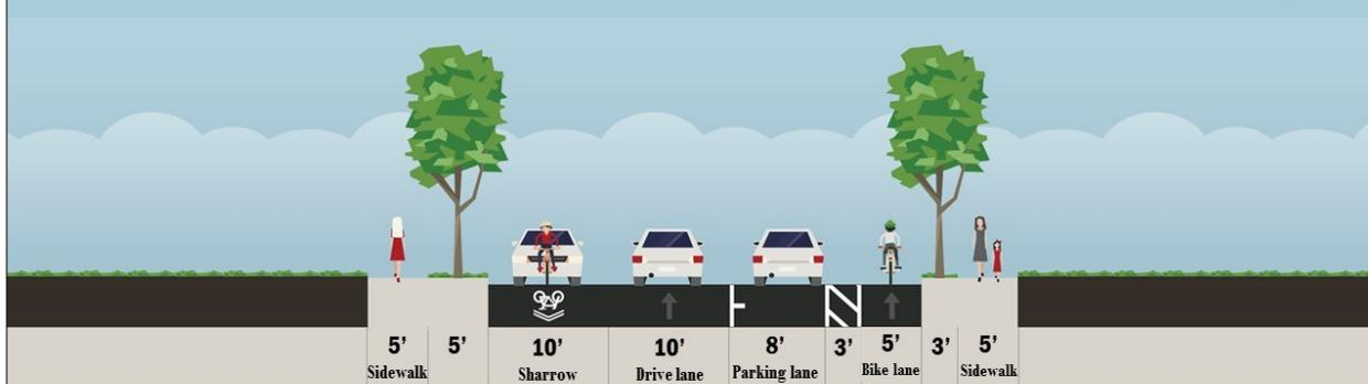
*Cross section showing existing conditions (top), and proposed improvements (bottom) including a new sidewalk on the west side, street tree buffer areas on both sides, a protected bike lane in the uphill direction, and sharrow markings in the downhill direction.*
