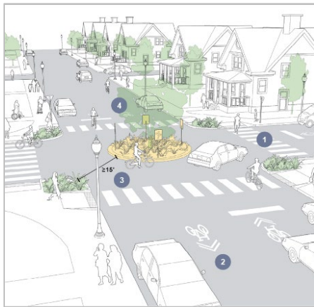
Mini-Roundabout (aka Traffic Circle) (source: NACTO)
