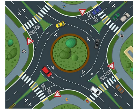
Multi-Lane Roundabout (source: FHWA)
