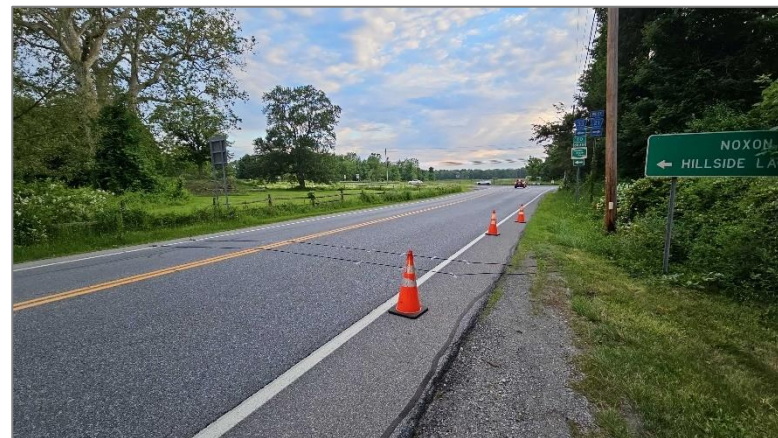
Our annual Traffic Count Program collects volume, classification, and speed data on a variety of county and local roads in Dutchess County, such as Noxon Rd in LaGrange shown here.
