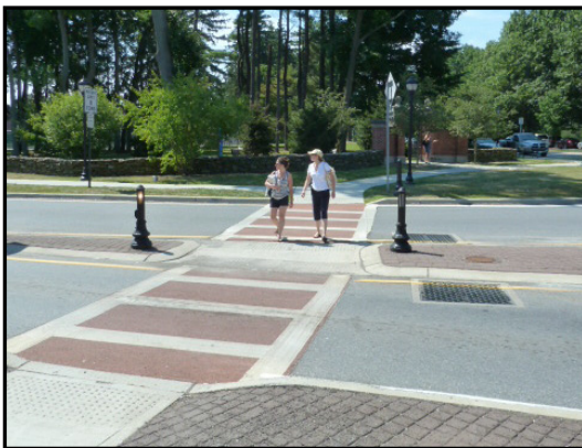
Arlington boasts wide, clearly marked crosswalks [left], and curb extensions that provide shelter for on-street parking while reducing the crossing distance for pedestrians in the crosswalk [right].
