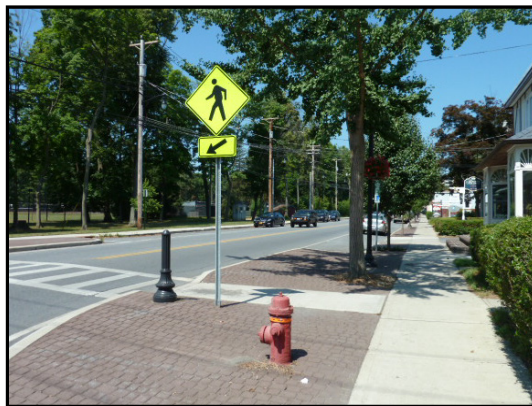
Arlington boasts wide, clearly marked crosswalks [left], and curb extensions that provide shelter for on-street parking while reducing the crossing distance for pedestrians in the crosswalk [right].
