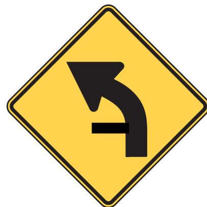
**Exhibit 22: Example of proposed combination alignment and intersection warning sign (W1-10).**
